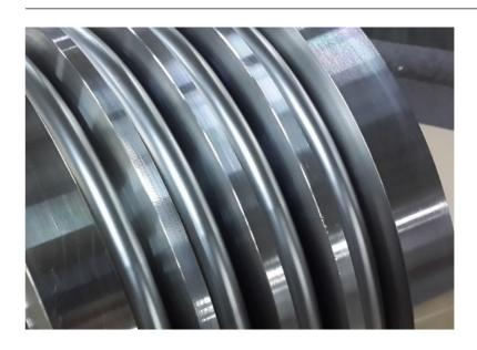
This DN200 expansion joint is designed for 130 barg for a mining facility. Expansion joint has weld ends and bellows has reinforcing rings to resist high pressure. All welds are dye penetrant tested by a Level II certified inspector and welded by certified welders. Completely designed, manufactured and tested by KLINGER Turkey.
